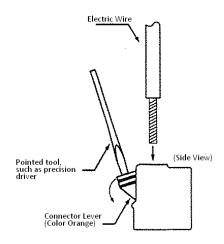
Insert the electric wire after pushing the connector lever inside as shown in the figure above. Pushing the electric wire inside with force without pushing the lever may lead to contact failure or disconnection.
